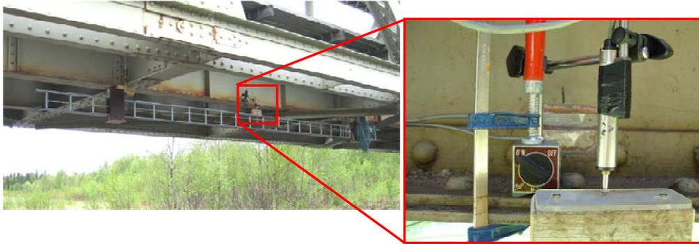
Figure 6.4 Arrangement of the cable rack underneath the bridge to provide a reference point to perform deflection measurement with a LVDT
